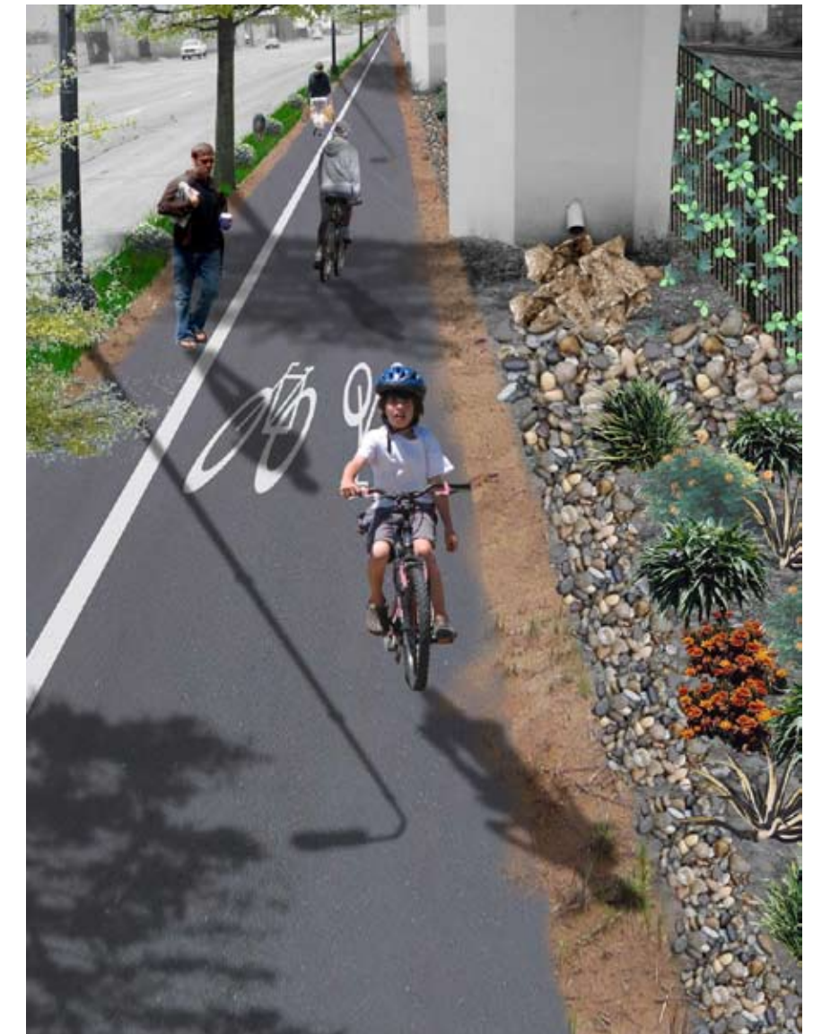
A simulation of splash rocks and a rain garden along the Greenway between the BART columns.
